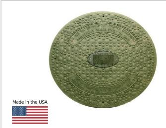
The Jackel Septic Tank Riser Cover is constructed of heavy duty structural foam. Utilizing our Tech Tough™ design technology, the cover can support up to 2,000 lbs. It comes with our molded, replaceable water tight seal. Insulation is an option for extreme climates. Each cover comes with our non-slip Lawn Deco™ decorative finish.
