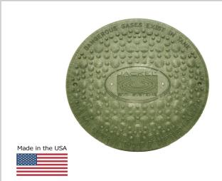
The Jackel septic tank riser cover is constructed of heavy duty structural foam. Utilizing our Tech Tough™ design technology, the cover can support up to 2,000 lbs. It comes with our molded, replaceable water tight seal. Insulation is an option for extreme climates. Each cover comes with our non-slip Lawn Deco™ decorative finish.
